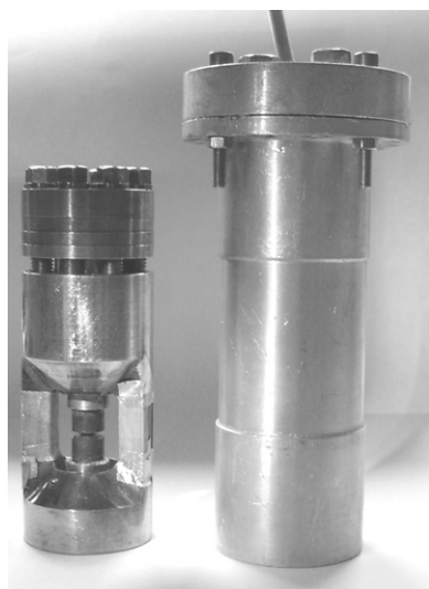
Figure 3. Left: the pressure cell with anvils made from cubic boron nitride. Right: the container used to load liquid oxygen into the cell.
